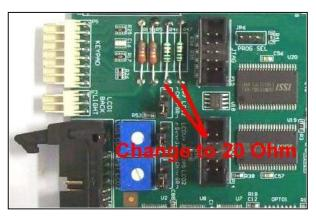
LM32019ECW-1 also has no contrast adjustment so potentiometer VR2 will be rendered obsolete.
